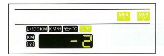
The multi-function indicator is equipped with two memories which operate independently of each other.
