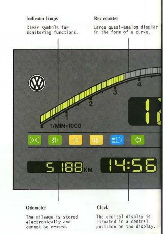
All displays and indicator lamps feature optimum design and can be read quickly. The display is illuminated from behind.
