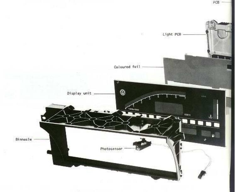
The binnacle, display unit and light PCB are grouped together to form one unit. The glass at the front is breakable. The display unit is connected to the PCB by means of an 8-pin connector.
