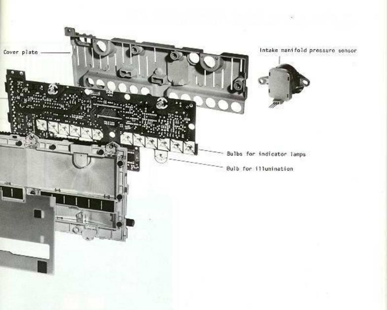
The PCB contains all electronic components, and a buzzer to provide an audible oil pressure indicator.
