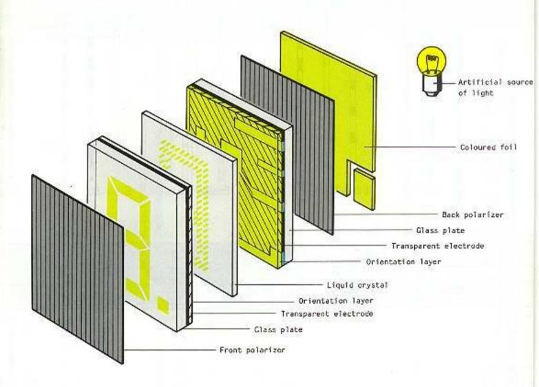
In the case of a digital display, each of the digits has 7 segments.
